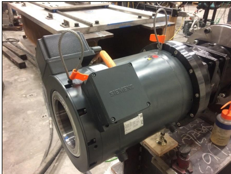
Figure 16: Siemens 1FW3 PMSM installed on the PTO test bench.
